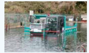
Transport robot for unmanned construction in the semi-submerged environment
